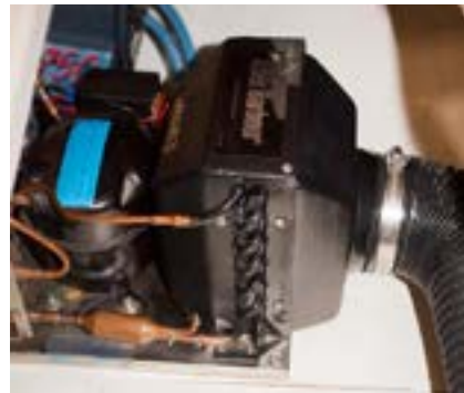
The condenser is sandwiched between fans, pushing airflow right to left.
