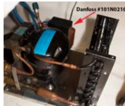
Housing and fans removed. Cooling fins on compressor controller pointing towards the airflow.
