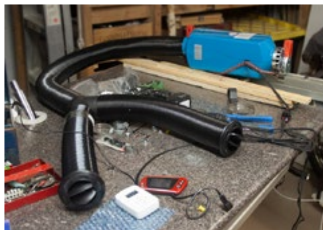
Bench testing the unit. Pairing the heater settings from the original (red) controller to the (white) Afterburner.
